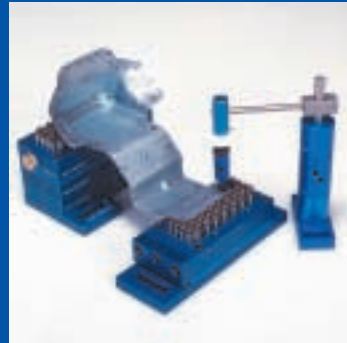
Correctly supported and fixed
