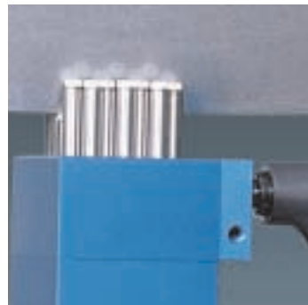
Pins with plastic caps for sensitive workpieces
