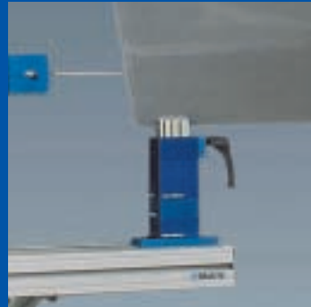
Pins with plastic caps for sensitive workpieces
